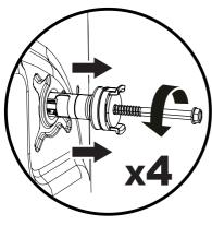
Transportation safety screws should then be removed by pulling them out. The removed transportation safety screws should be stored to be used again in case the machine needs to be transported again, e.g. if moving house.
